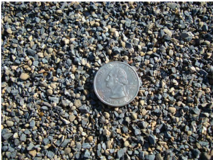
Calcined bauxite is the most commonly used HFST aggregate (Image: David Merritt)
