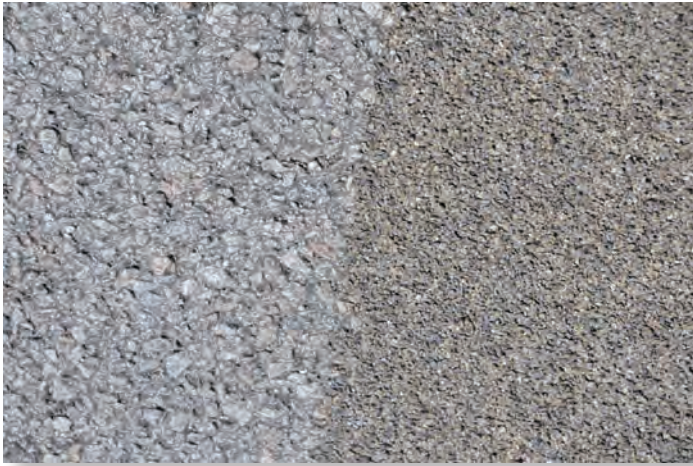
HFSTs (right) provide additional surface microtexture (Image: South Carolina DOT)
