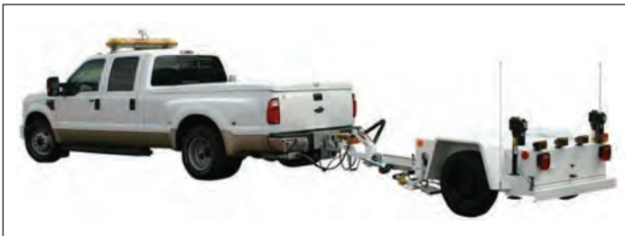
Locked wheel skid trailers are the most commonly used friction measurement device (Image: International Cybernetics)
